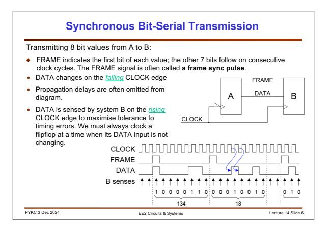
Let us consider two systems A and B, and we want to send digital data between them. The obvious method is to send the digital data one bit at a time. Such serial communication method has many advantages: 1) It is very simple to do; 2) it only needs very few wires linking between the two systems.
