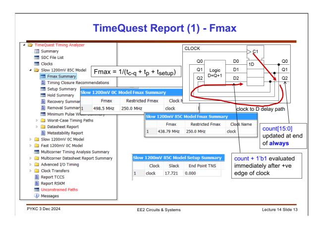
If you implement this on the Cyclone III FPGA, you can use the **timing analyser**, known as **TimeQuest**, in Quartus to work out the timing constraints for you. This reports that the maximum operating frequency of the counter is 498.5MHz. However, due to the limitations of the pins, the maximum observable frequency is 250MHz. This is because the pins and pads of the chip is rather slower than the internal logic.
