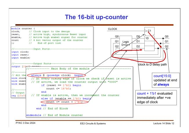
Now let us consider the Verilog specification for a 16-bit up-counter. The red arrows here indicates the delay paths from the rising edge of the clock to the Q output, then through the logic block D=Q+1 and you must also add in the setup time of the flipflop.
