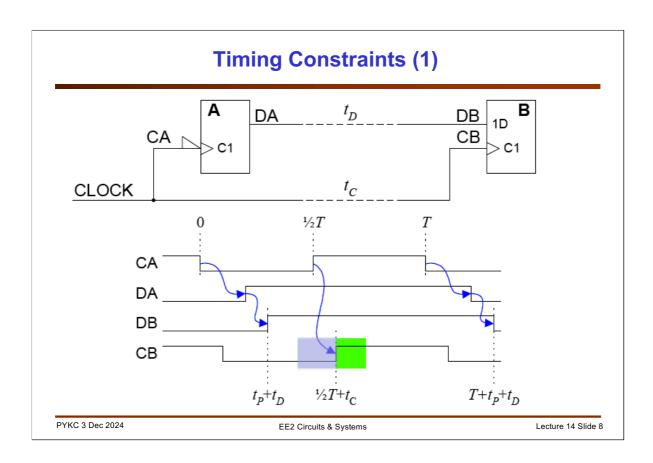
In order to guarantee reliable working of the serial interface circuit, the rising edge of CB must become stable outside the setup time window (shown in light blue).
