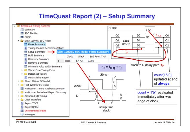
For this circuit, it also reports the timing slack. We are running the clock at 20ns period or 50MHz. Then the setup time slack is 17.721ns. That is D settles to its final value 17.721ns earlier than it is required.
