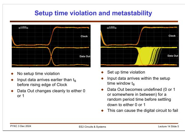
The waveforms shown here illustrates what happens when setup time violation occurs. The Data Out signal becomes indeterminate for a period of time before settling down to either 0 or 1.
