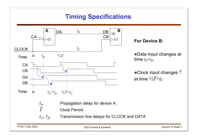
Here is the timing diagram for the data travelling from A to B via a synchronous serial link. CA is the clock signal to module A. It also supply CB, but CB is delayed by  $t_{\rm C}$  due to the propagation from A to B.
